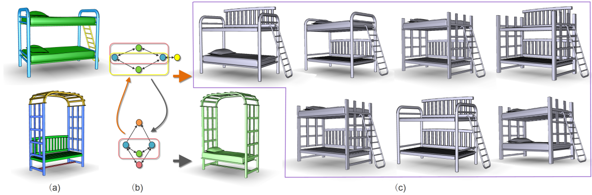
Figure 2: Algorithm overview. Given two (pre-segmented) shapes (a), we extract and encode mutual part relations (e.g., symmetry, contact, and support) in the form of relation graphs (b). Next, certain compatible symmetric functional arrangements (SFARR) are detected in each graph (shown by boxes in both graphs) and subsequently reshuffled to produce model variations. Note that even two models can produce dozens of variations (c), yet the synthesized models remain plausible.
