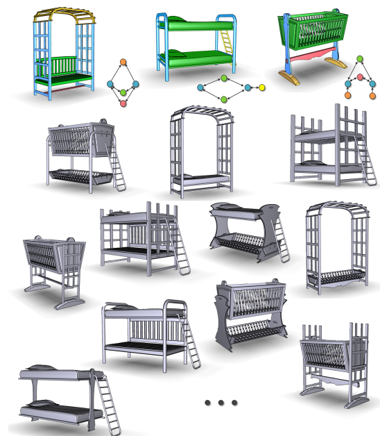
Figure 1: Starting from only three models (top), our algorithm detects and exploits symmetric functional arrangements (SFARR-s) to generate more than 20 variations. Many of the variations have strong geometric differences, but still preserve the object sub-structures and functionalities.
